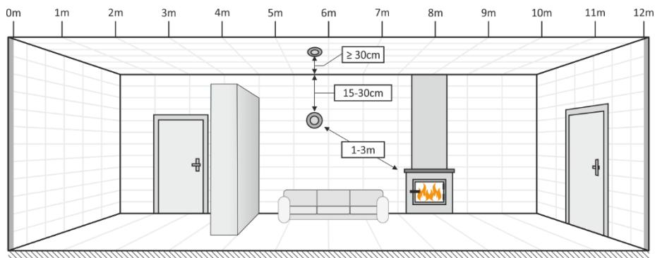
**NOTE: Never place a carbon monoxide detector in the following locations:**
