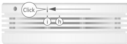
After approximately 60 seconds, the carbon monoxide alarm has fully booted up. Next, check if the device is functioning properly by pressing and holding the test/mute button for approximately 3 seconds. If the device is working properly, it will beep four times and flash red. If this is not the case, do not use the device and contact the supplier.
